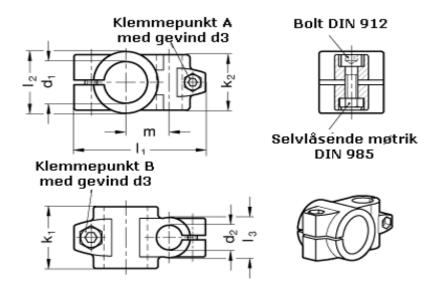
Adjustable clamp lever for d3 = GN 911-M 8-32 have to be ordred separately Adjustable clamp lever for d4 = GN 911-M 6-25 have to be ordred separately d1 = 30
